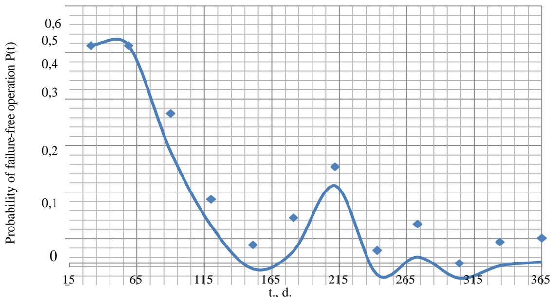
Fig. 3. Dynamic changes in probability of failure-free operation  $P(t)$  under normal distribution of the failure rate
