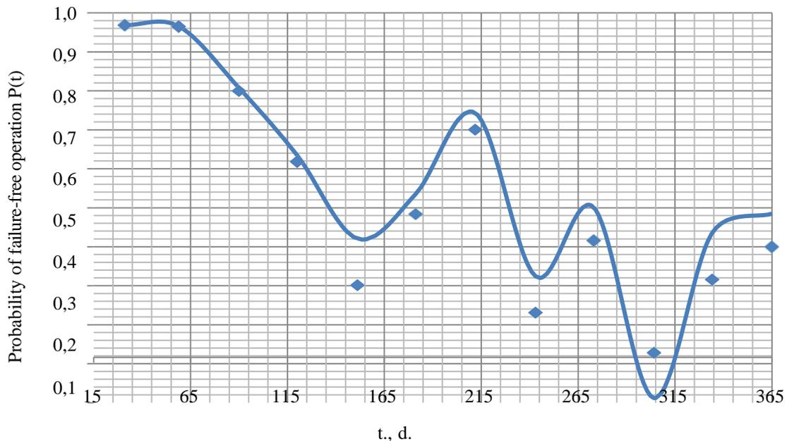
Fig. 2. Dynamic change of probability of failure-free operation  $P(t)$  under exponential distribution of the failure rate
